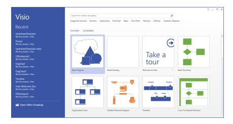
Each template includes shapes related to the type of drawing, in specialized collections called stencils. The **Shapes** window, at the side of the drawing, holds the most popular stencils and shapes for the diagram type you're making.
